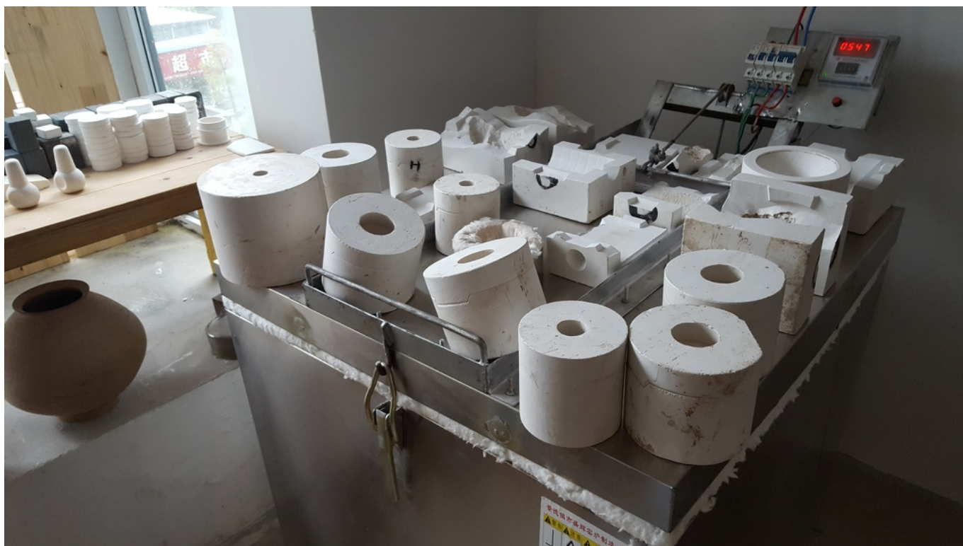
High humidity slows the process of molds drying, so they're often stacked around kilns. Christy just had these made.
