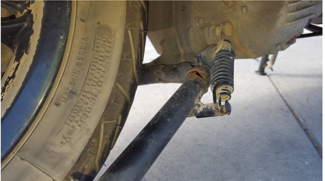
Tear in the center stand. Definitely not going to hold any weight. Note the spring is beyond the tear. Cause for future excitement.
